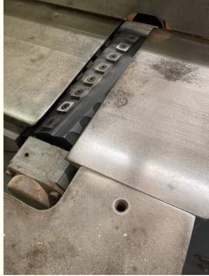
A Look At The Newly Installed Helical Cutter Head And The Refurbished Rockwell / Delta Jointer!
