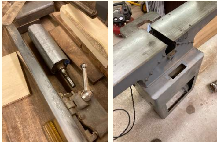
The Old Cutterhead (Left) & Jointer Without Cutterhead (Right)
