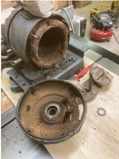
A Look At A 1940 GE 3/4 HP 120 V Motor With 82 Years Of Dust & Dirt Buildup. Amazing It Still Works!
